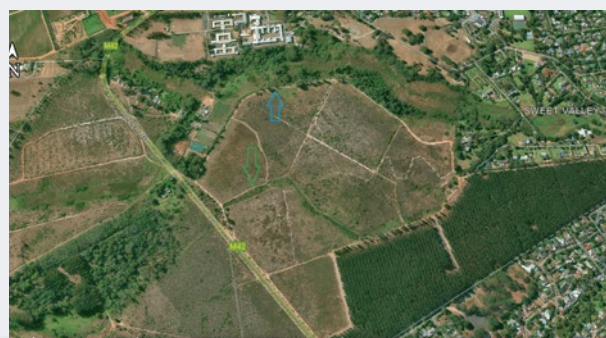
River channel historically re-aligned from natural watercourse (blue arrow) to make way for forestry, resulting in a perched channel (green arrow) and drying out of natural wetlands.
